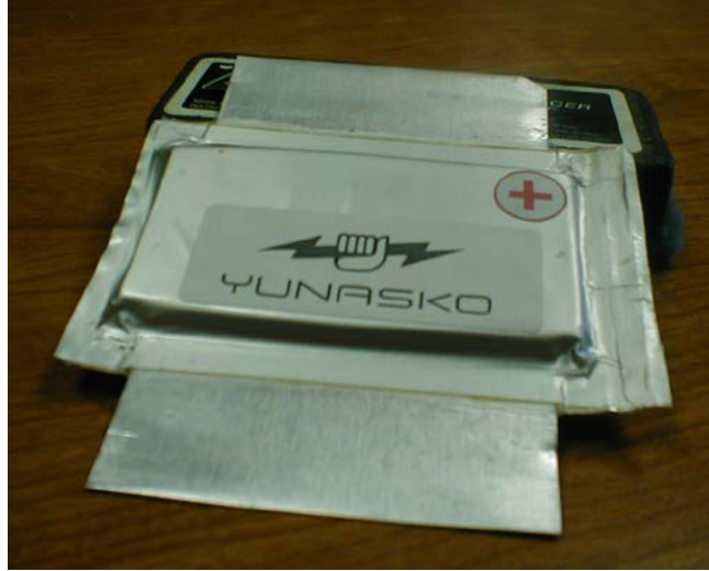
Figure 5: Photograph of the 5000F Yunasko Hybrid ultracapacitor 5000F device
