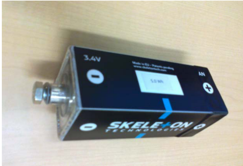
Figure 3: Photograph of the 3200F Skeleton Technologies device
