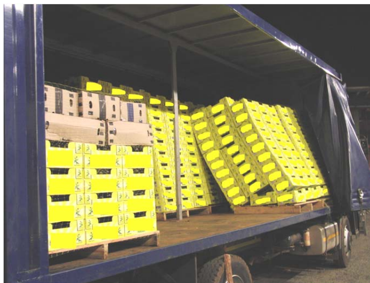
Figure 5.11: Typical damage to fresh produce cargo due to road roughness.
