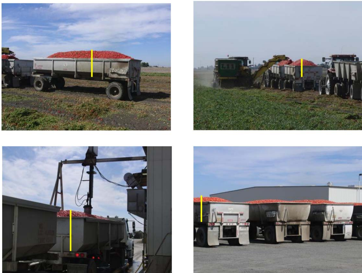
Figure 4.11: Visual indication of densification of tomato cargo during transport.
