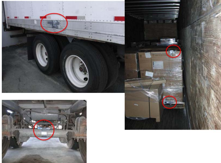
Figure 3.23: Company B accelerometer detail.
