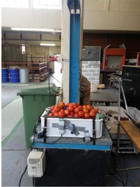
Figure 5.5: Vibration table with tomatoes in container ready for testing.
