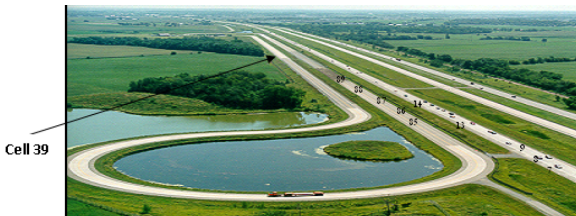
Figure 2. MnROAD Test Facility and Cell Location Cell 85 = pervious concrete on sand, cell 86 = porous asphalt on sand, cell 87 = pervious controls, cell 88 = porous asphalt on clay, cell 89 = pervious concrete on clay, cell 39 = pervious concrete overlay. (Izevbekhai and Akkari 2011).
