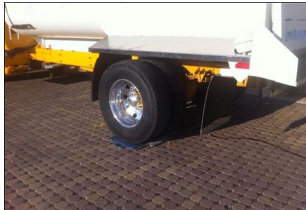
Figure 2.5: Measuring the wheel load.
