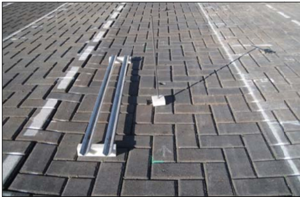
Figure 6.8: Permanent deformation measurements.
