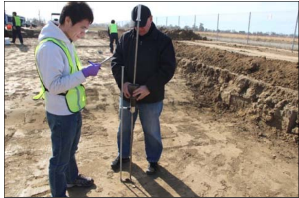
Figure 5.6: Dynamic cone penetrometer measurements.
