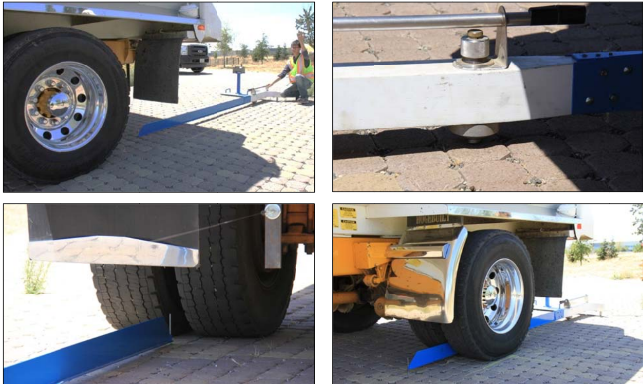
Figure 2.1: Road surface deflectometer.
