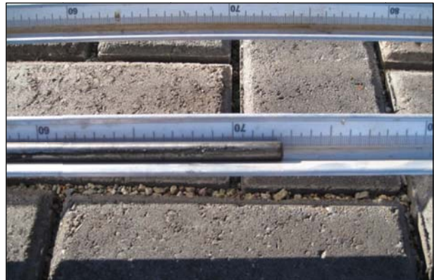
Figure 6.8: Permanent deformation measurements.
