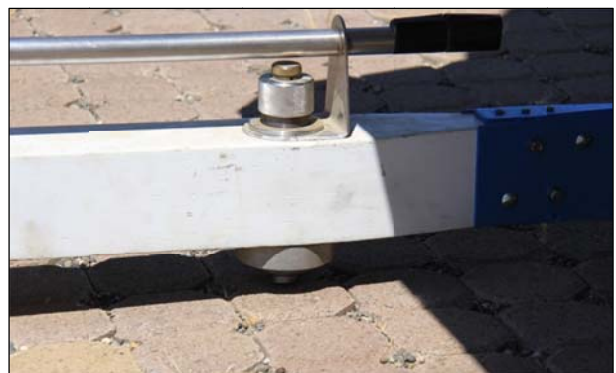
Figure 6.9: Road surface deflectometer.
