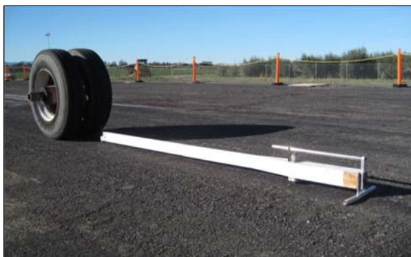
Figure 6.9: Road surface deflectometer.
