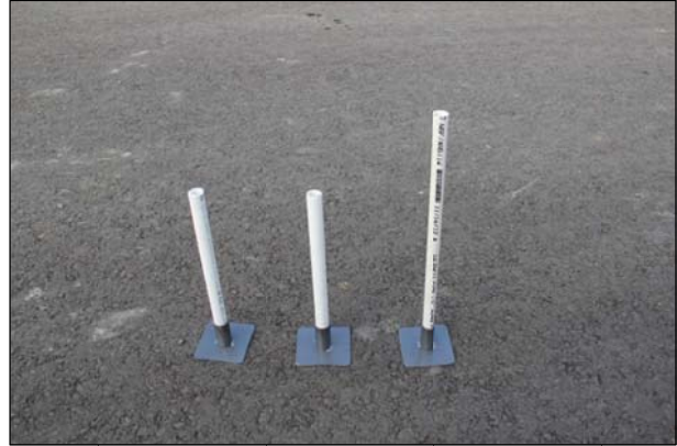
Figure 6.7: Permanent deformation gauge.
