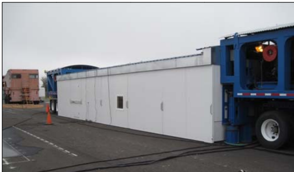
Figure 1.3: HVS with environmental chamber.
