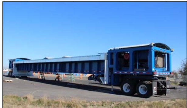
Figure 1.4: Heavy Vehicle Simulator with extended beam.
