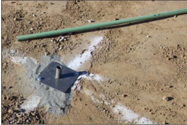
Figure 6.7: Permanent deformation gauge.
