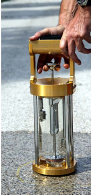
Figure 3.3: Outflow meter. (Courtesy of KLARUW Systems)
