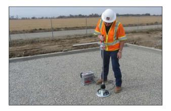
Figure 3.2: Light weight deflectometer.
