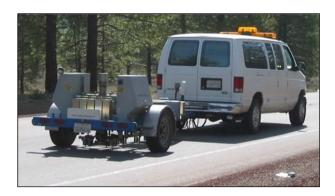
Figure 3.1: Falling weight deflectometer.
