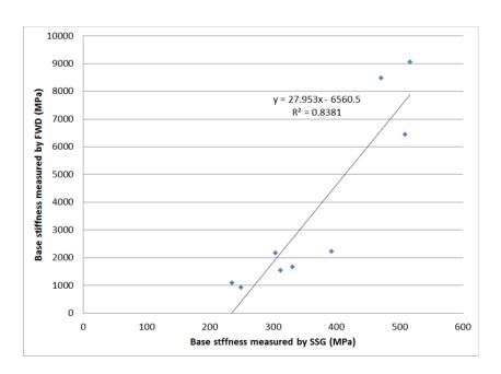
Figure 3.5: Relationship between FWD and SSG measured stiffness (25).
