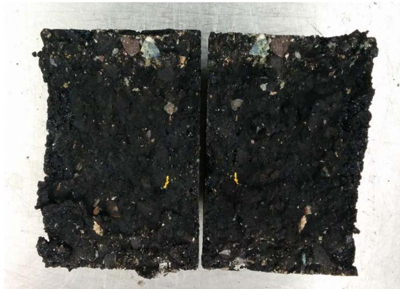
**Figure 2.19 Post-test IDT specimen exhibiting fractured aggregate.**
