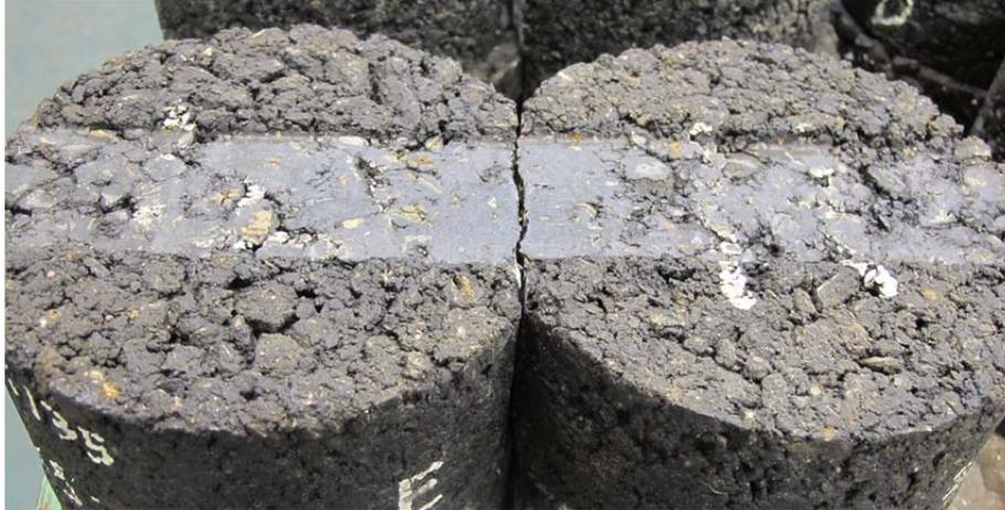
Figure 2.16: HMA cores following HWTT testing.
