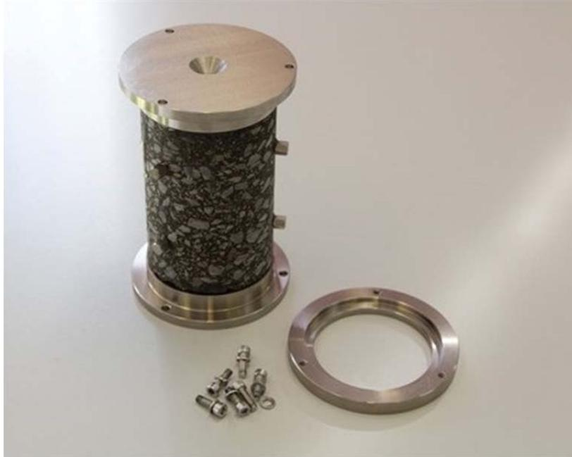
Figure 2.13: AMPT direct tension fatigue test specimen and end caps (end caps glued to specimen).
