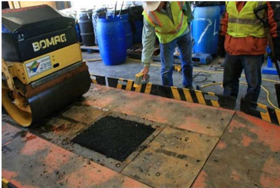
**Figure 2.24: HMA specimen production by rolling-wheel compaction.**
