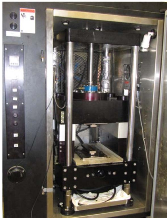
Figure 2.4: Simple shear testing machine.
