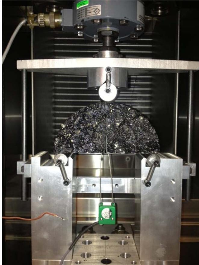
**Figure 2.20: SCB test apparatus with specimen under test.**
