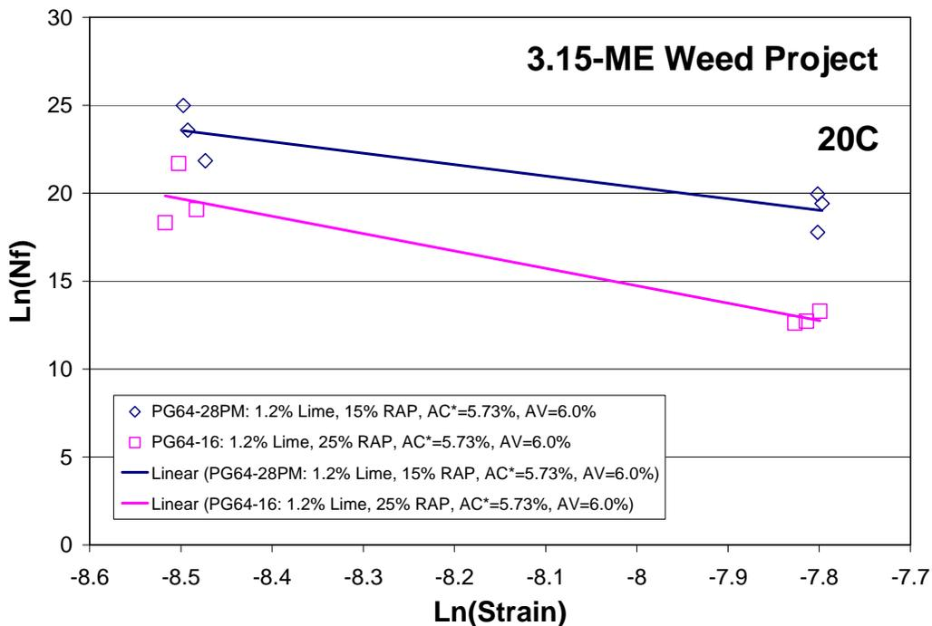
Figure 4.2: Fatigue test summary for the Weed Project.
