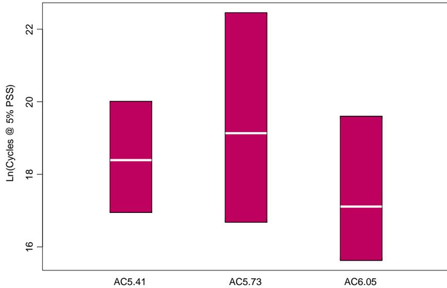
Figure A.3: Ln (repetitions at  $\gamma_p = 5\%$ ) versus binder content, Weed PG 64-28PM, 15% RAP, 1.2% lime mix (50°C, 70 kPa stress).
