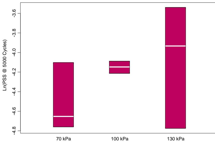
**Figure A.6:  $\ln(\gamma_p @ 5000 \text{ Cycles})$  versus stress level, PG 64-28PM 15% RAP, 1.2% lime mix (ME, Weed Project, AC = 5.73%, 50°C, LMLC).**
