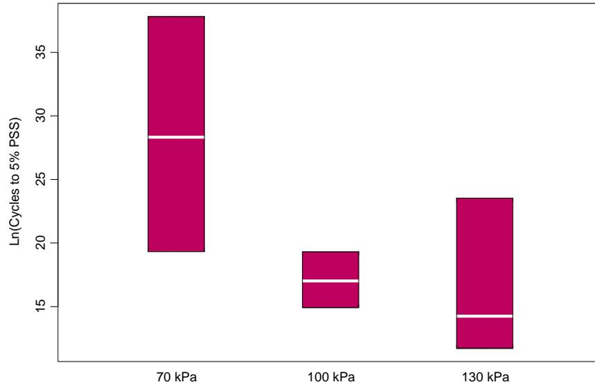
**Figure A.7: Ln (load repetitions to  $\gamma_p = 5\%$ ) versus stress level, PG 64-28PM 15% RAP, 1.2% lime mix (ME, Weed Project, AC = 5.73%, 50°C, LMLC).**
