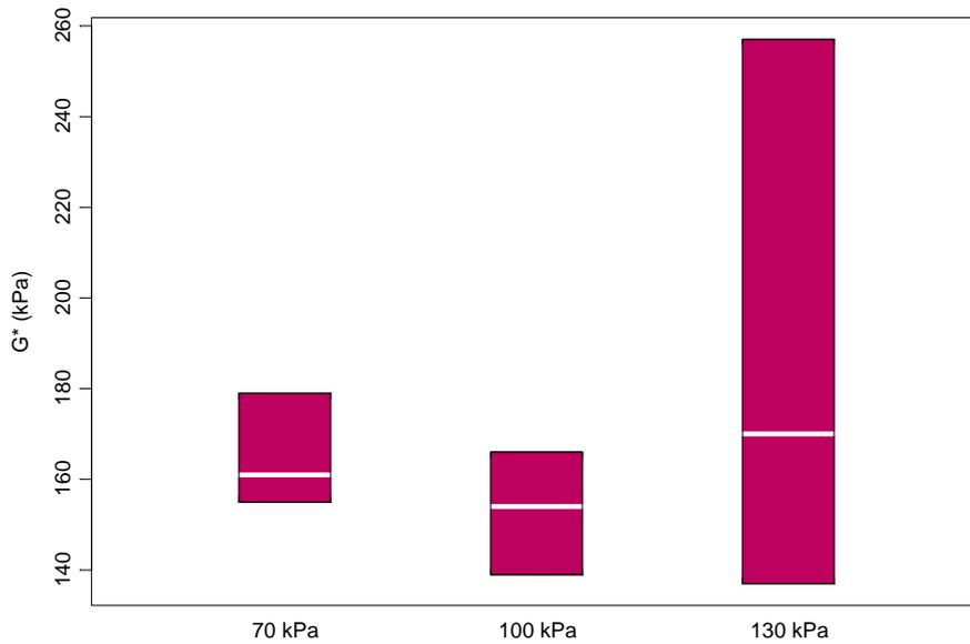
**Figure A.5:  $G^*$  versus shear stress level, PG 64-28PM mix (ME, Weed Project, AC =5.73%, 15% RAP, 1.2% lime, 50°C, LMLC).**
