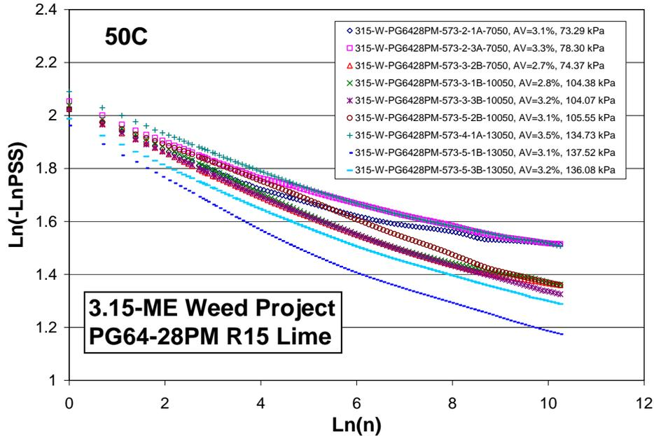
Figure A.4: Summary of shear test results, Ln ( $L_n \gamma_p$ ) versus Ln (load repetitions), PG 64-28 mix (ME, Weed Project, AC = 5.73% [by weight of virgin aggregate plus lime], 15% RAP, 1.2% lime, AV = 3.0%, LMLC).
