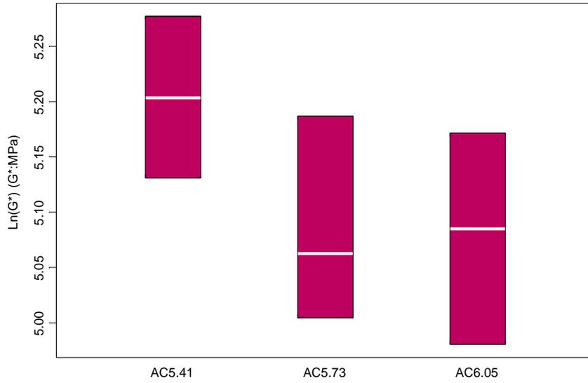
Figure A.1: Ln (G) versus binder content, Weed PG 64-28PM, 15% RAP, 1.2% lime mix (50°C, 70 kPa stress).
