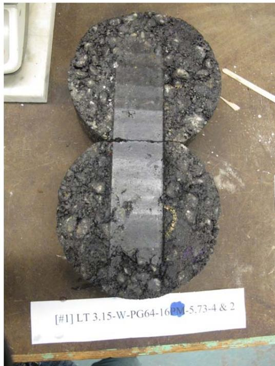
**Figure C.6: HWTT result for PG 64-16 25% RAP, 1.2% lime (set #1 lt.) after 40,000 passes.**
