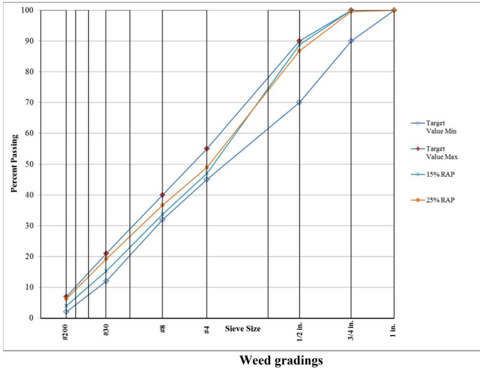
**Figure 2.1: Aggregate gradings with 15 percent and 25 percent RAP.**
