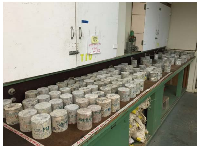
Figure 2.10: Concrete pavement cores after cutting and leveling for strength testing.
