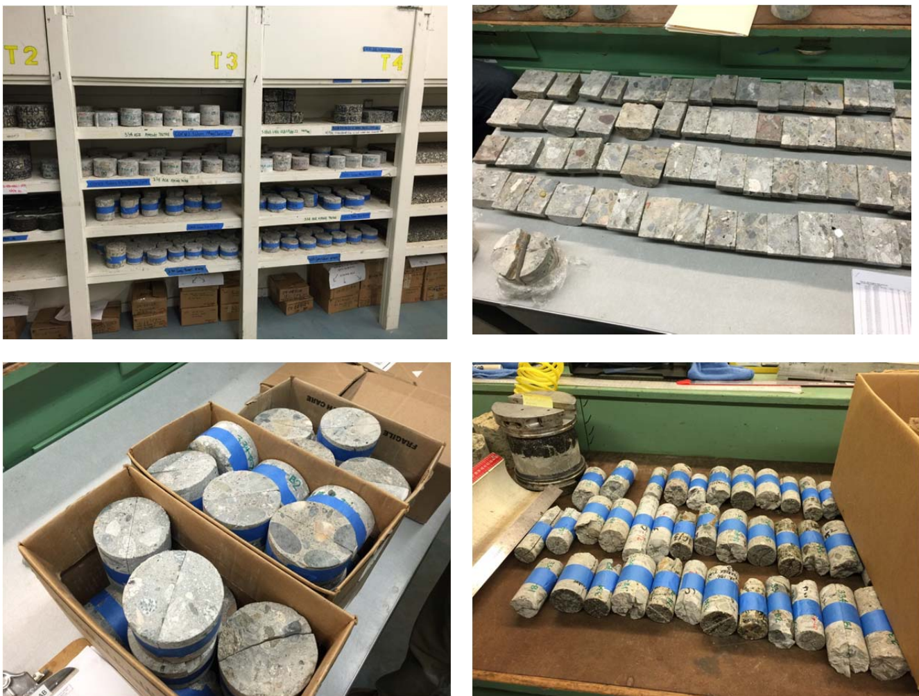
Figure 3.1: Pavement and bridge cores after cutting for visual inspection.
