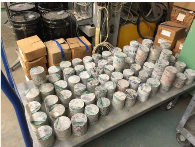
Figure 2.10: Concrete pavement cores after cutting and leveling for strength testing.
