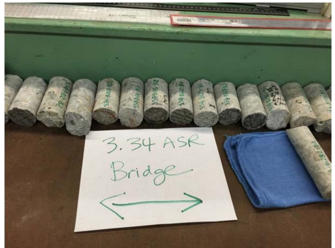
Figure 2.9: Concrete cores for visual inspection.
