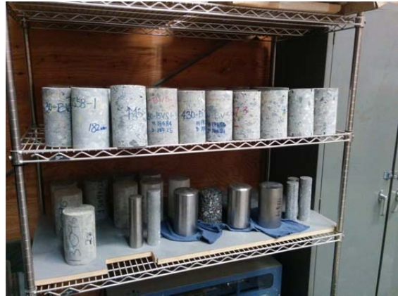
Figure 2.1: Pavement cores, including 150 cores that had been soaked in lime water for CTE testing.
