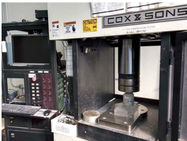
Figure 4.1: Pavement cores and strength testing.
