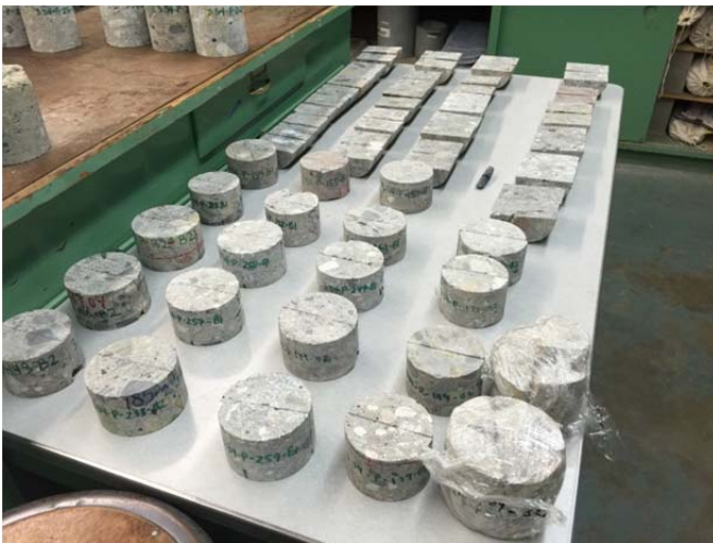
Figure 2.9: Concrete cores for visual inspection.
