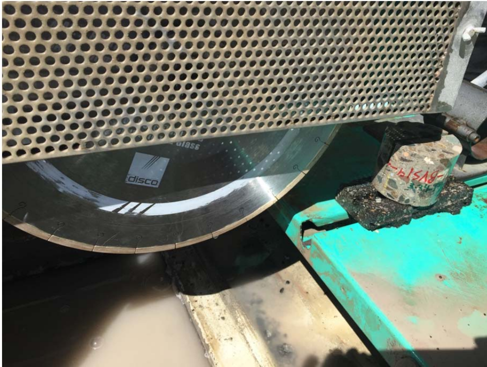
Figure 2.7: J-slot continuous diamond blades for concrete core cutting.
