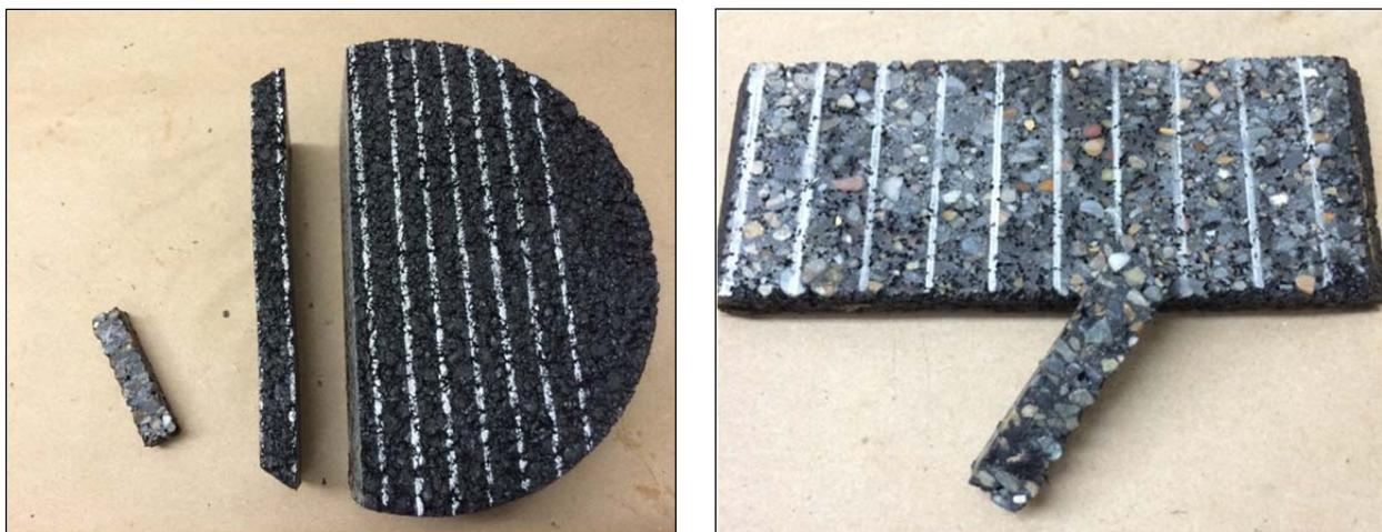
**Figure 4.2: Cut FAM mix specimens (asphalt rubber binder).**
