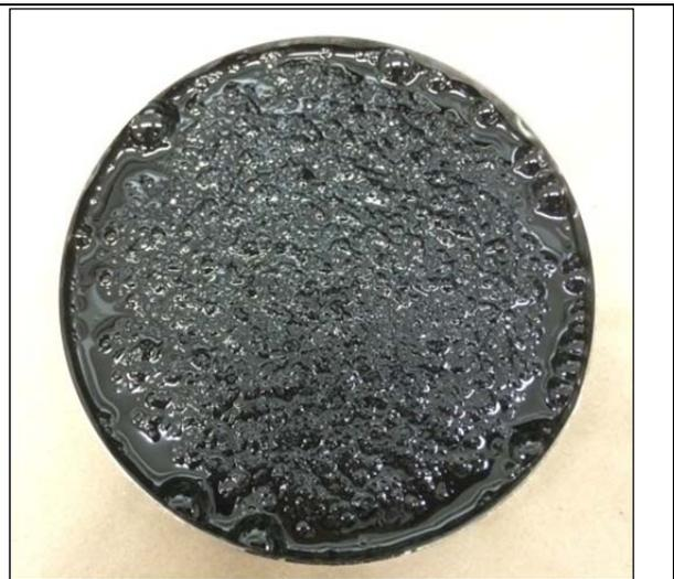
**Figure 5.4: PAV-aged sample.**
