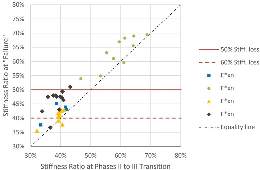
Figure 3.18: Stiffness ratio at failure, according to the three failure criteria (50 and 60 percent stiffness reduction and maximum of  $|E^*| \times n$ ).
