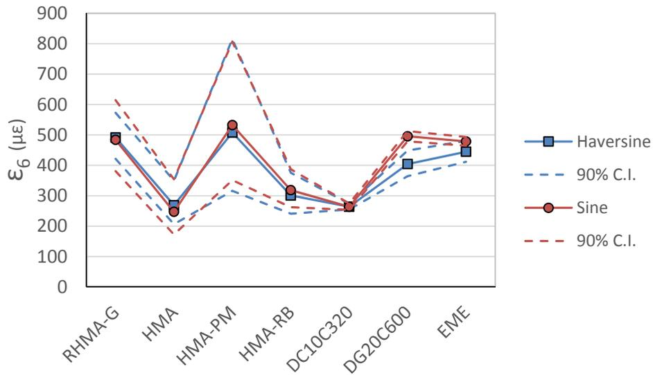
**Figure 3.6: Strain (peak-to-peak) corresponding to a fatigue life of 10<sup>6</sup> cycles (50% stiffness reduction failure criterion).**
