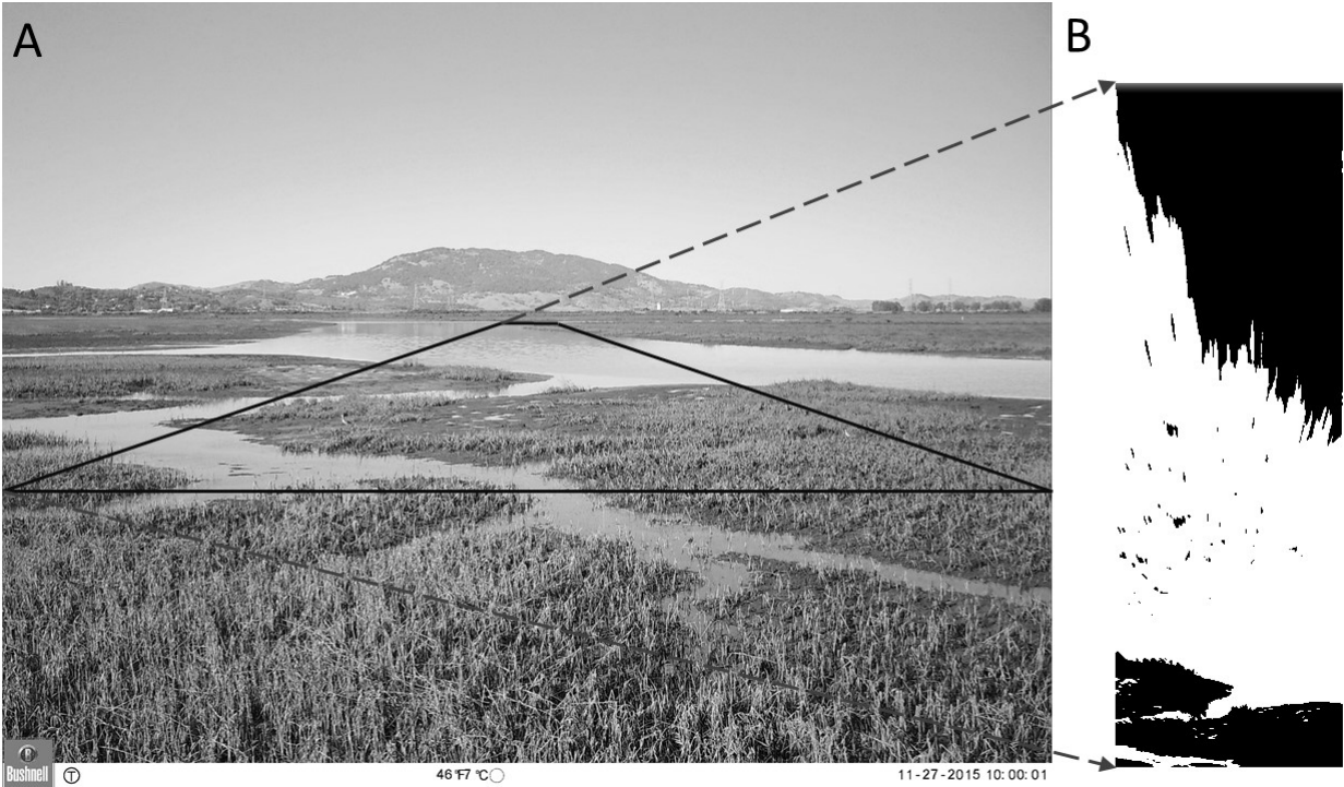
FIGURE 2. Correction for perspective and conversion to image for quantification of water surface area. A) Trapezoidal area used to select sample area within image for correction. B) Resulting rectangular sample area, converted to 2-colors (black and white), where white corresponds to water surfaces.
