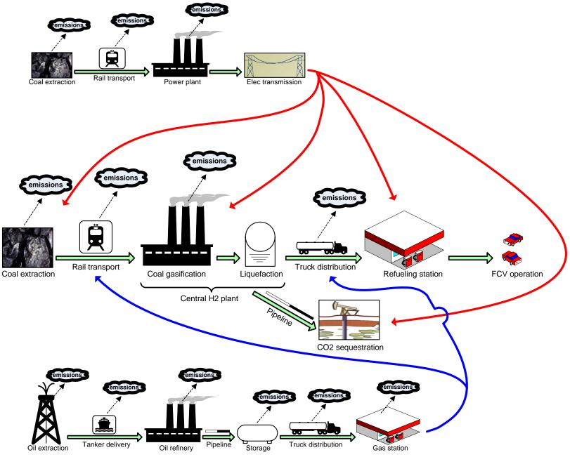
6. Coal-to-H2 pathway (Liquefied H2) with electricity and petroleum input
