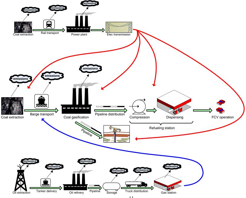
3. Coal-to-H2 pathway (pipeline) with electricity and petroleum input (and electricity input to petroleum)
