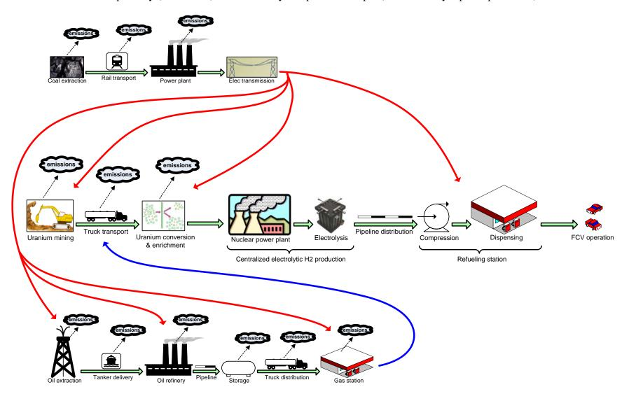
14. Uranium-to-H2 pathway (centralized) with electricity and petroleum input (and electricity input to petroleum)
