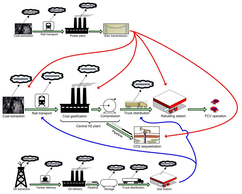
4. Coal-to-H2 pathway (compressed H2) with electricity and petroleum input
