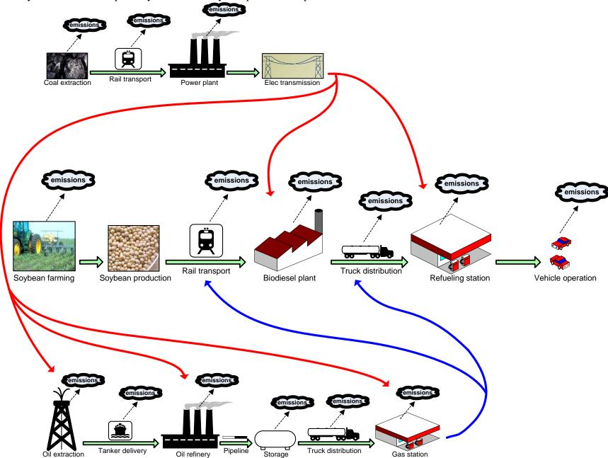
16. Soybean-to-biodiesel pathway with electricity and petroleum input:
