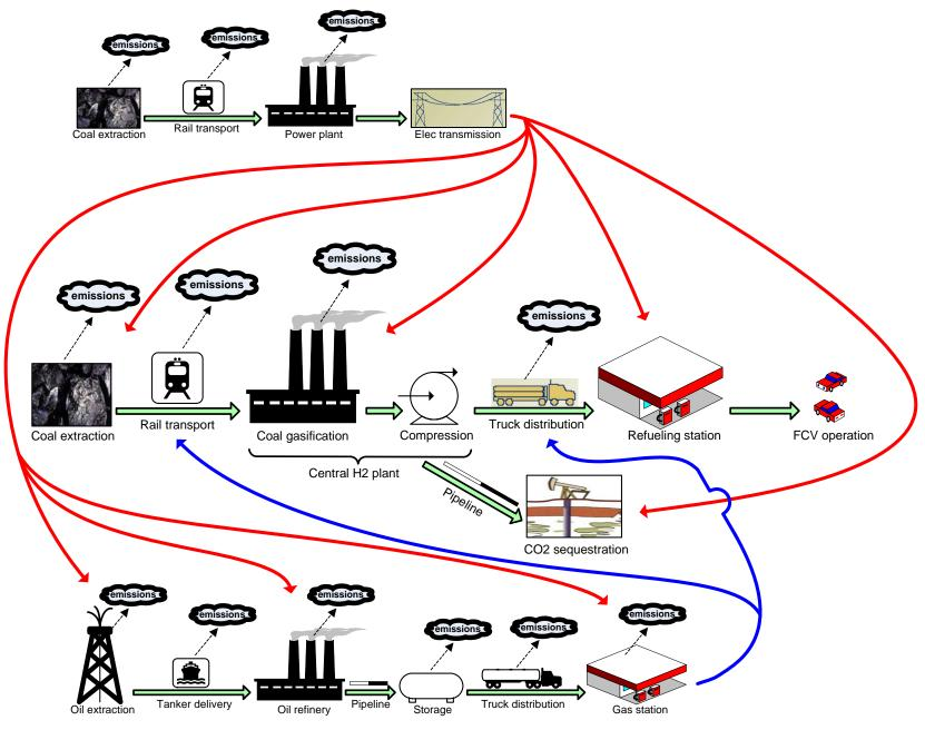
5. Coal-to-H2 pathway (compressed H2) with electricity and petroleum input (and electricity input to petroleum)
