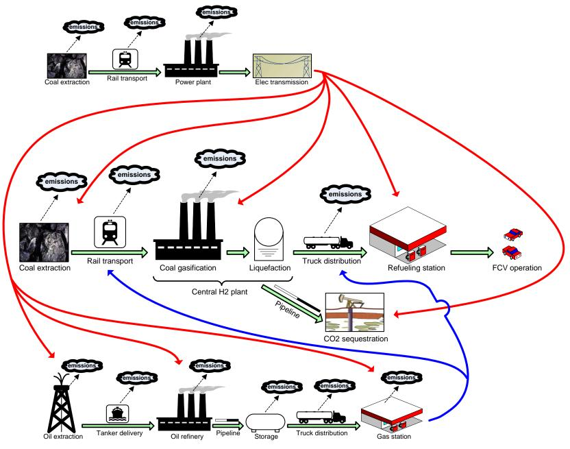
7. Coal-to-H2 pathway (Liquefied H2) with electricity and petroleum input (and electricity input to petroleum)
