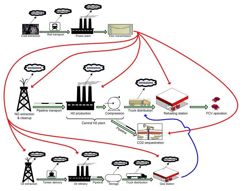
10. NG-to-H2 pathway (compressed H2) with electricity and petroleum input (and electricity input to petroleum)
