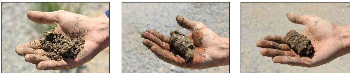
Figure 5.5: Squeeze test for assessing moisture content.
