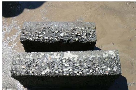
(b) Slab samples, porous part is the CIR layer
