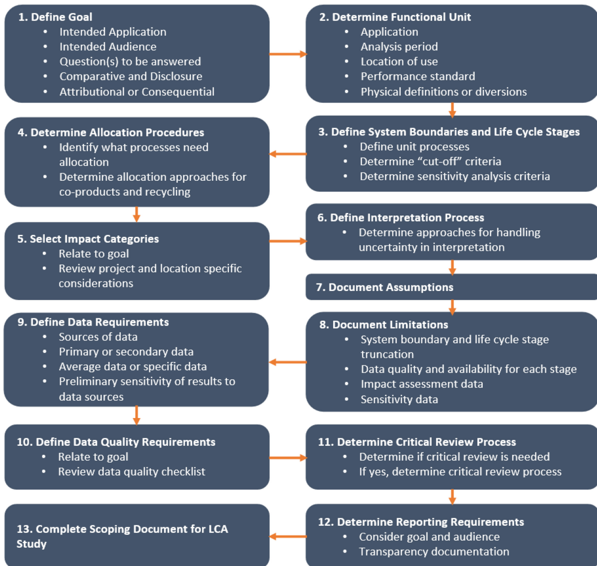
Figure 3-1. Flow chart for developing goal definition and scoping document for LCA studies.
