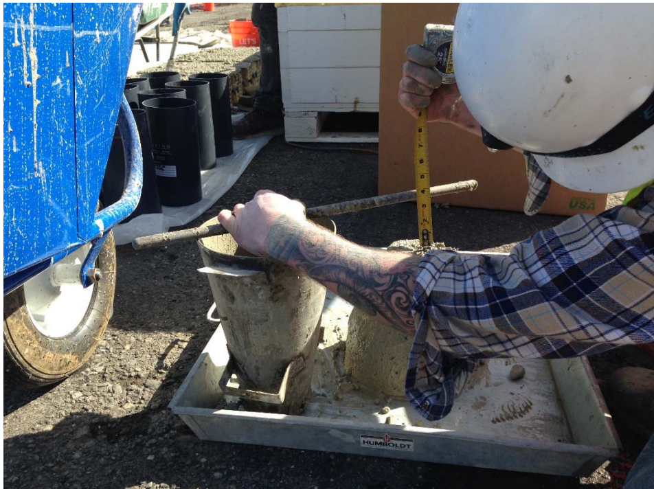
Figure A.62: Slump test measurement.
