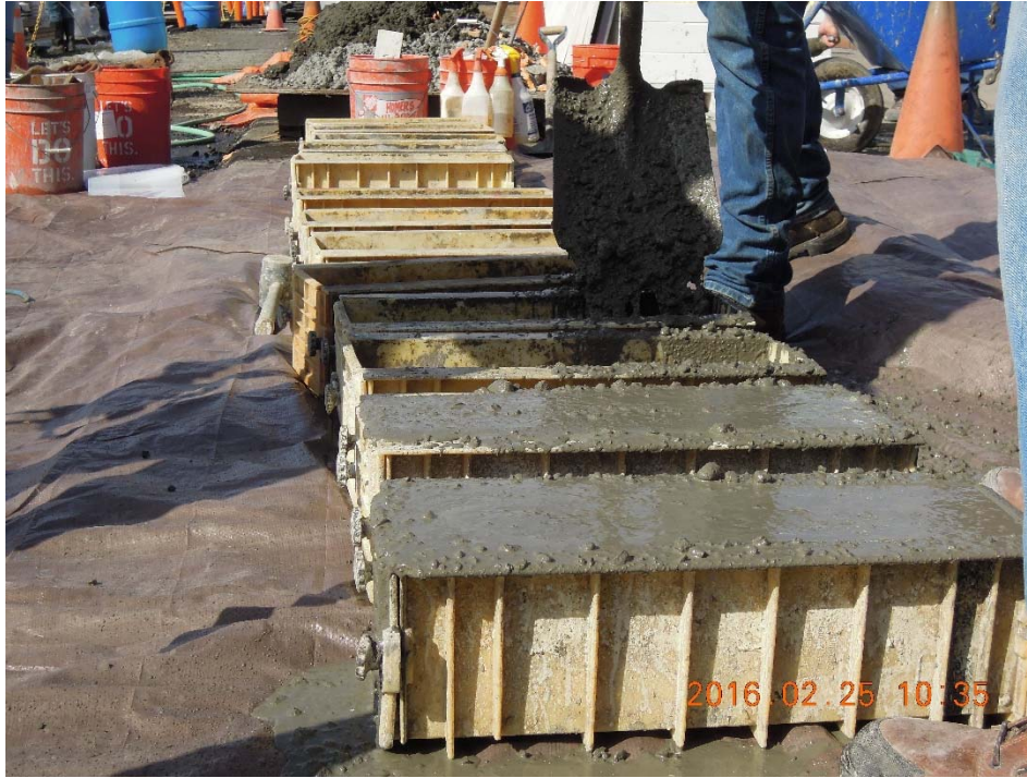
Figure A.87: Flexural beam preparation.
