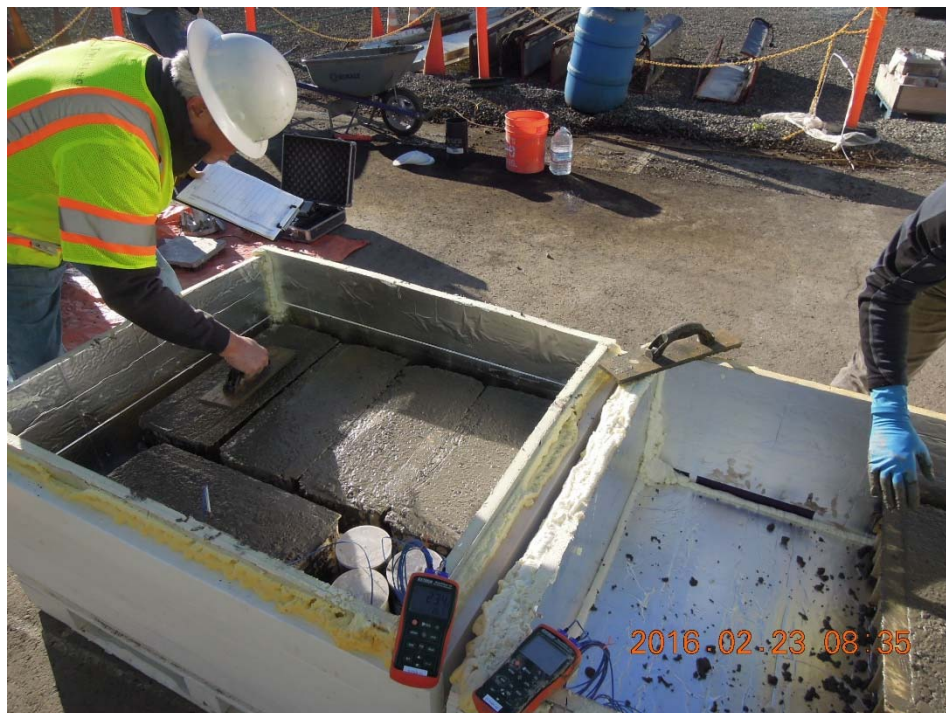
Figure A.46: Concrete beams inside insulated curing boxes.
