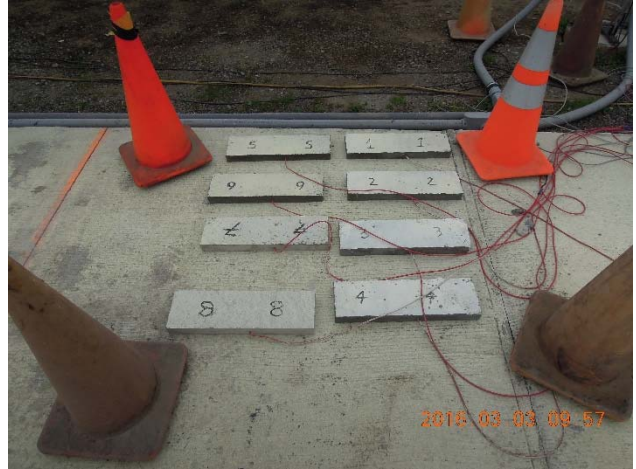
Beams after demolding
