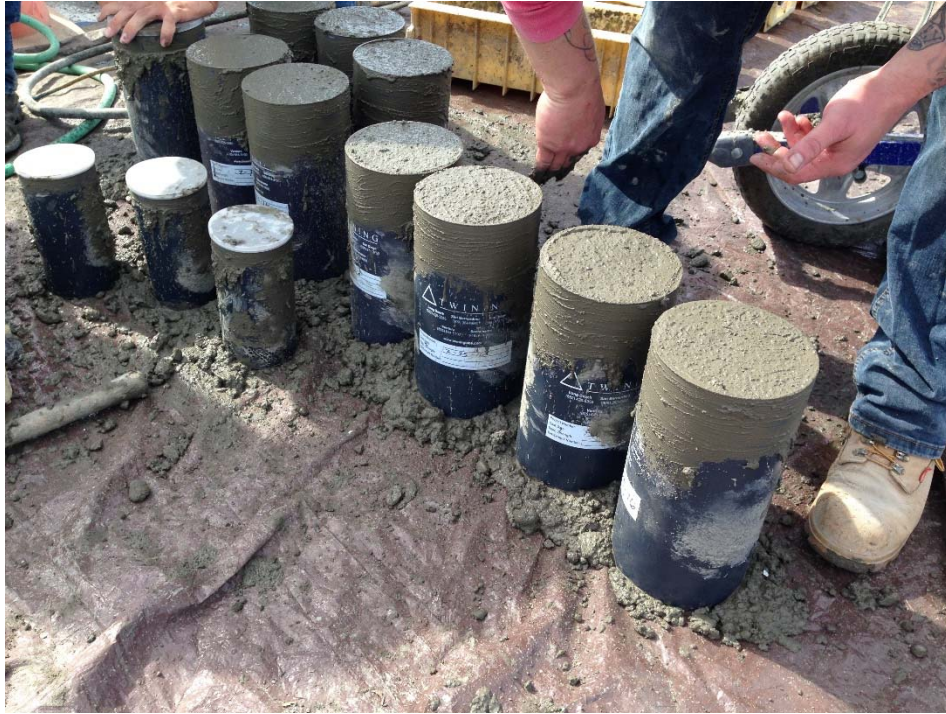
Figure A.95: Concrete cylinders for compressive strength, modulus of elasticity, and CTE testing.
