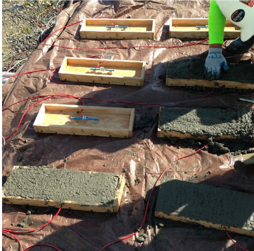
Figure A.89: Unrestrained shrinkage beams.
