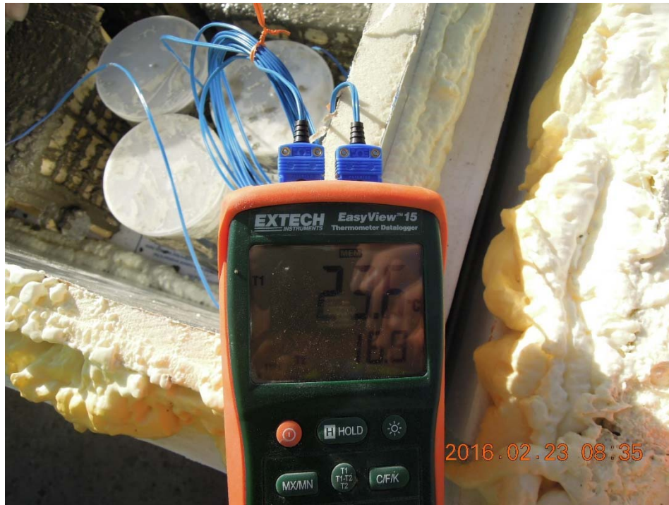
Figure A.47: Temperature tracking inside beams and cylinders.
