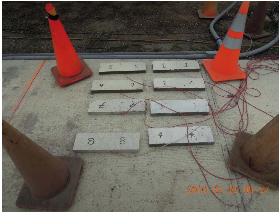
Figure A.109: Unrestrained shrinkage beams.
