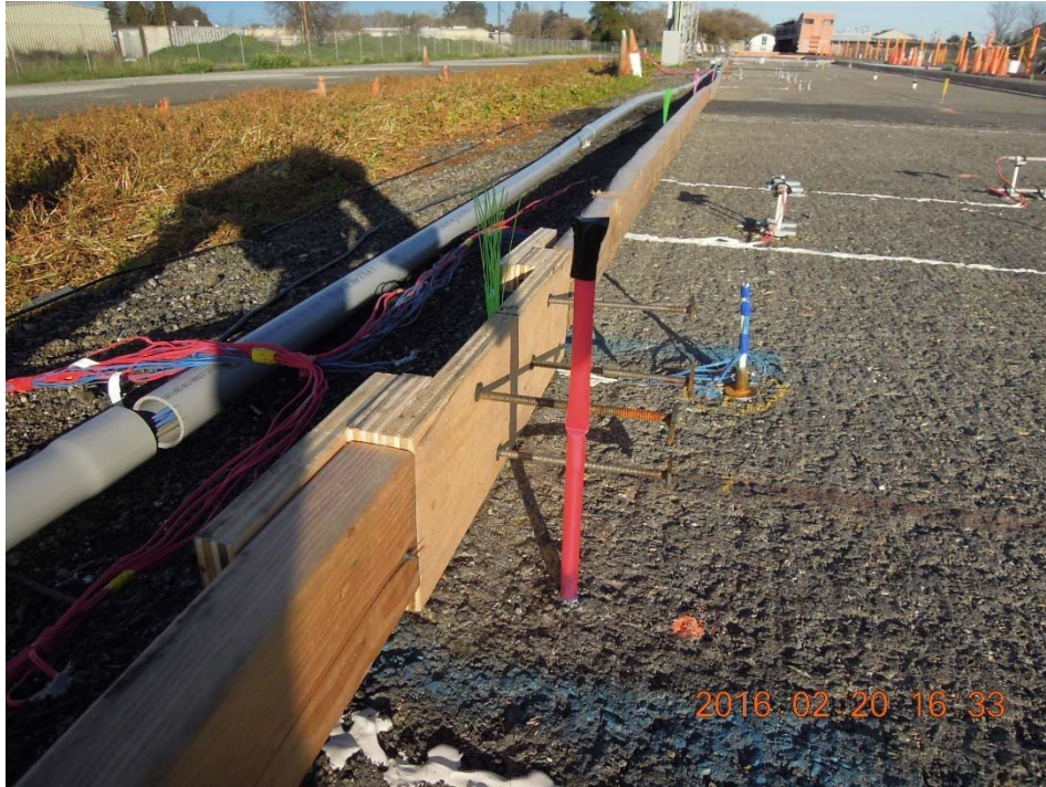
Figure A.17: Close-up of thermocouple rods and rod of IOMD protected by red straw.
