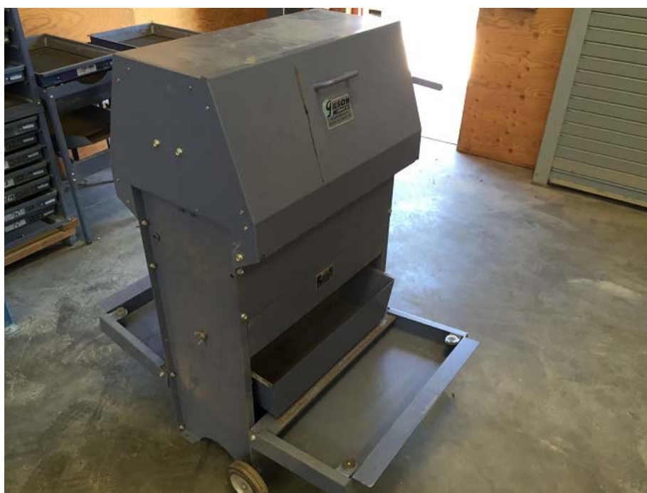
Figure A.4: Large enclosed sample splitter.
