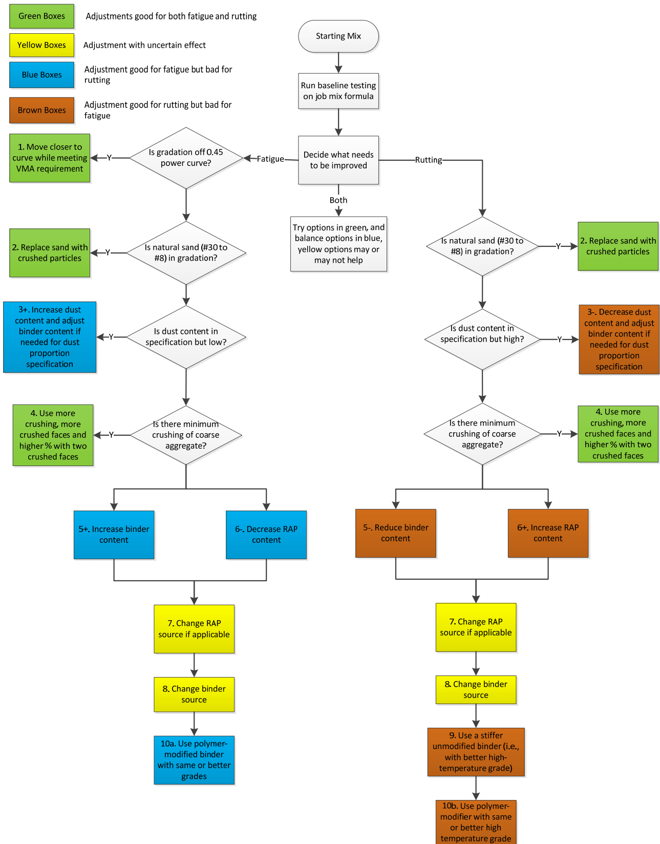
Figure 9.1: Revised flowchart proposed for improving the fatigue or rutting performance of an HMA mix.
