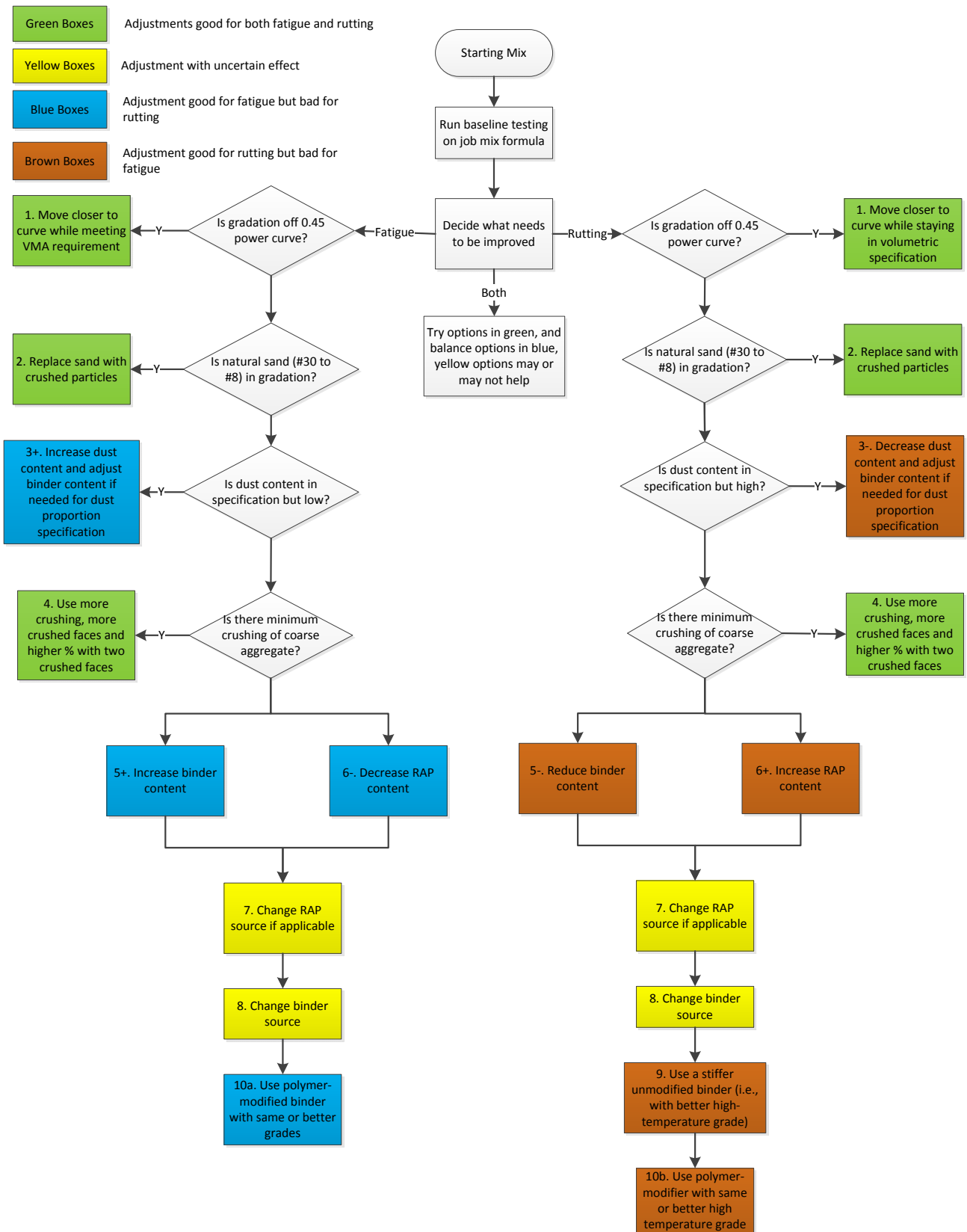
Figure 2.1: Initial flowchart proposed for improving the fatigue or rutting performance of an asphalt concrete mix.
