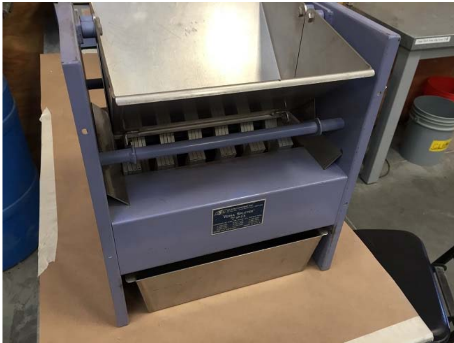
Figure A.5: Small sample splitter.
