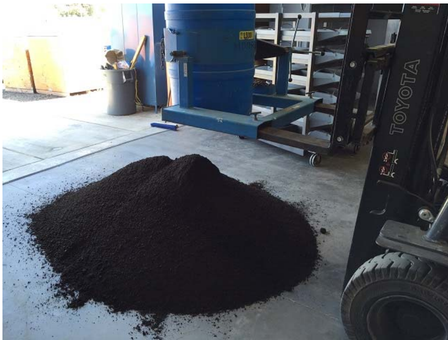
Figure A.1: Example conical sample pile on a hard, clean, level surface.
