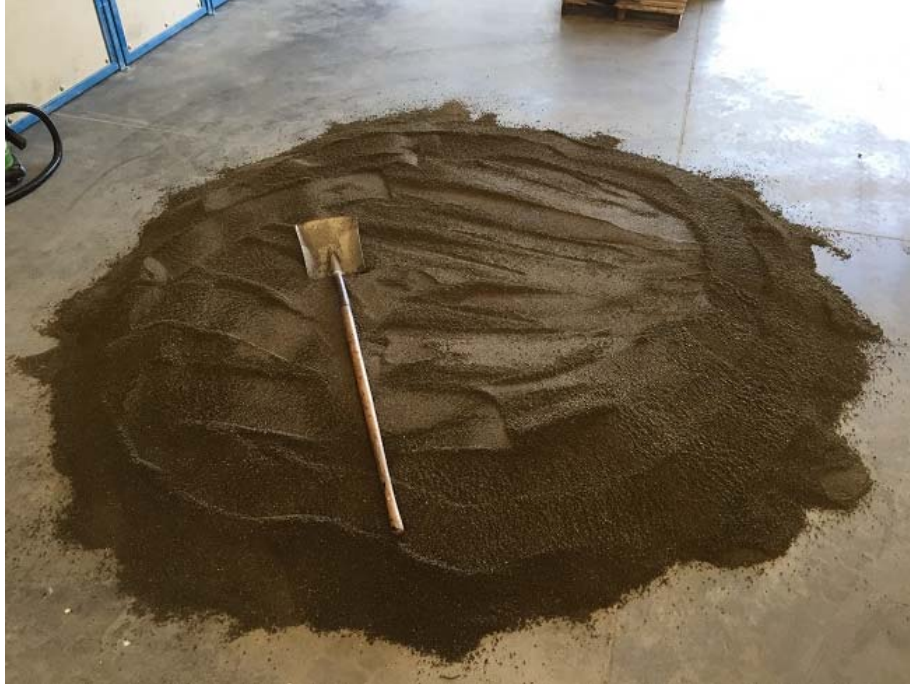
Figure A.2: An example of blended and flattened conical pile.
