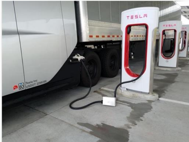
A photo taken in January of 2019 and uploaded to Facebook shows the Tesla Semi truck charging connector, possibly for the first time publicly. Photo credit: Joseph Mathew
