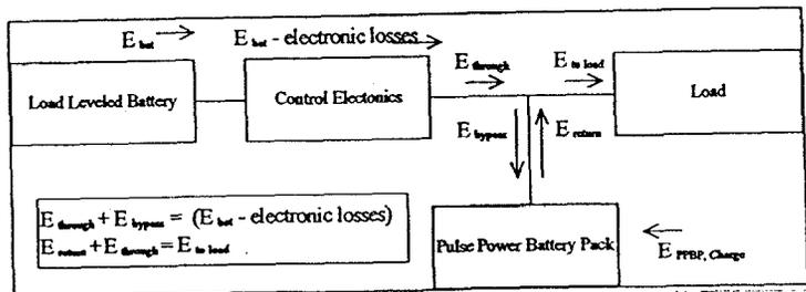
Figure 6: Schematic of Energy Flow in the Load Levelled Battery System
