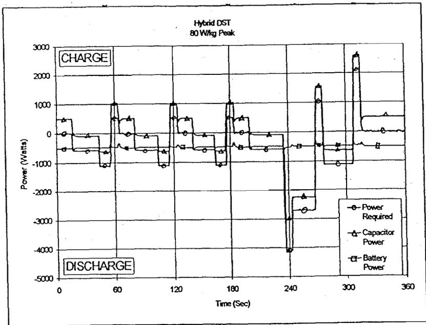
Figure 5: Power Profiles for the Energy Battery and Pulse Power Unit on the DST Cycle
