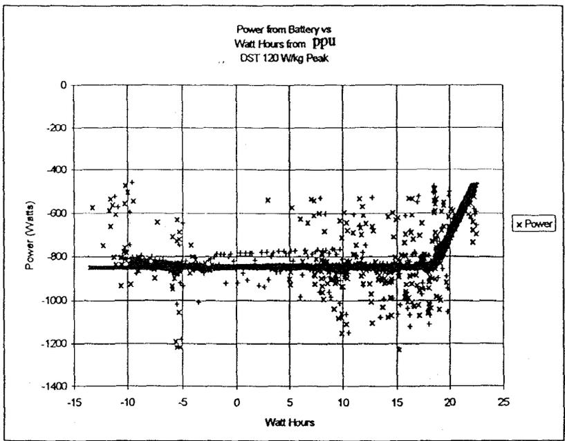
Figure 4: Load Levelled Battery Power Test Data
