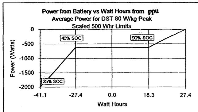
**Figure 3: Control Strategy - Load Leveled Battery Power vs. Pulse Power Unit SOC**
