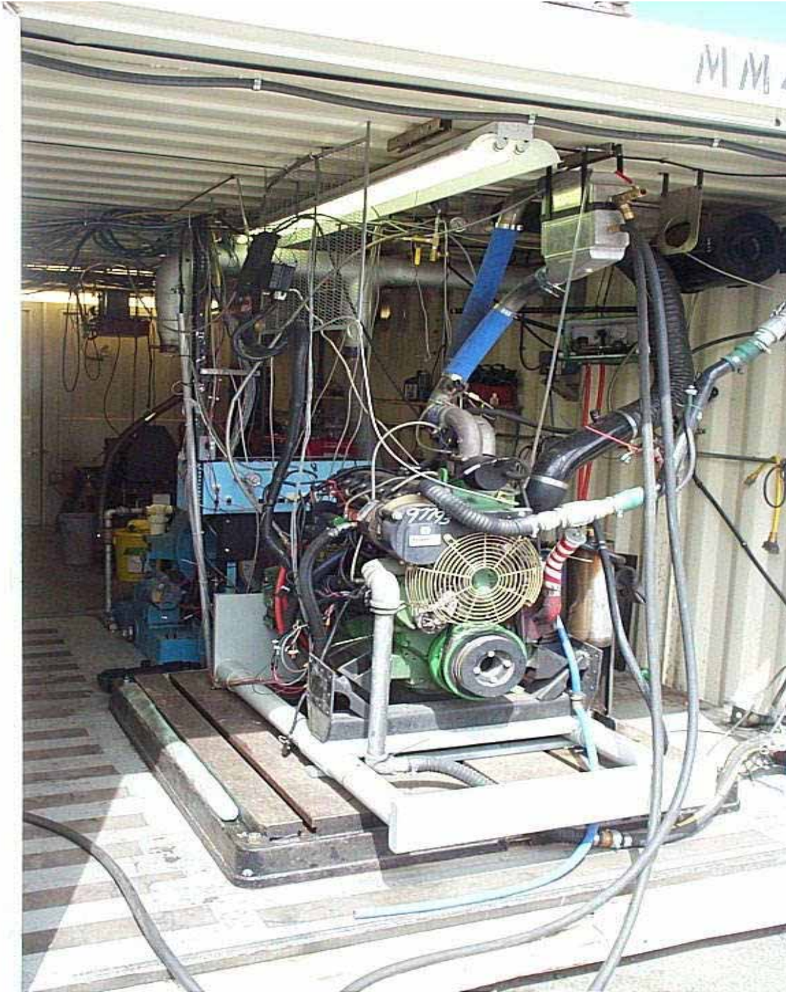
Figure 1. The Phase II modified HCNG engine on the Collier Technologies dynamometer.
