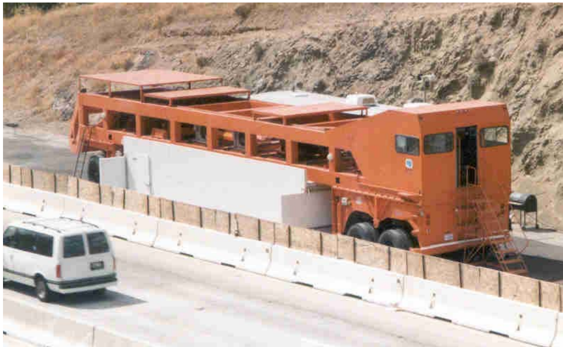
Figure 1-4. Heavy Vehicle Simulator with temperature control chamber (from du Plessis, 2002B).
