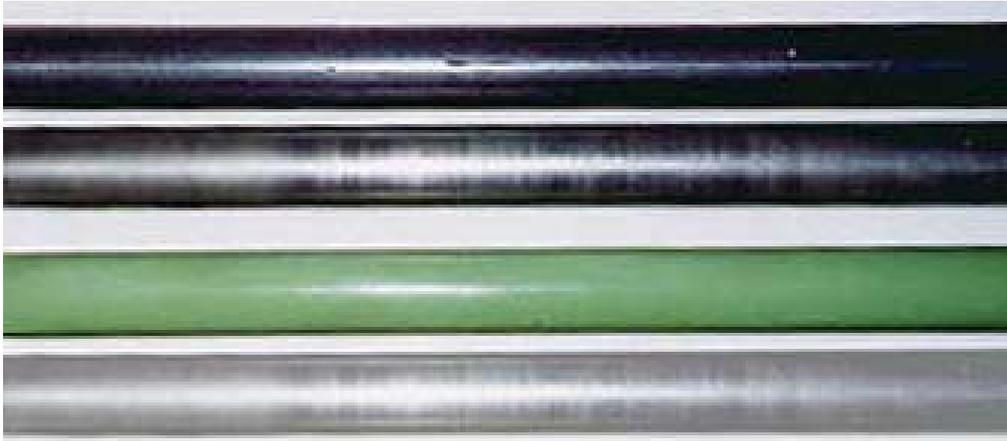
**Figure 3. Steel dowel types investigated in Phase I. From top to bottom: carbon steel, stainless steel clad, carbon steel coated with bendable epoxy, and stainless steel hollow.**
