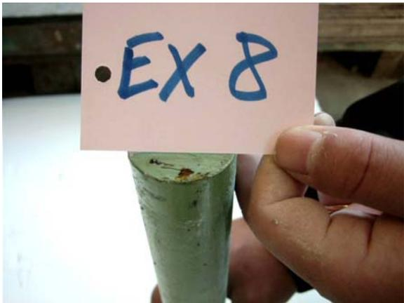
Figure 23. Corrosion on the epoxy-coated bars.
