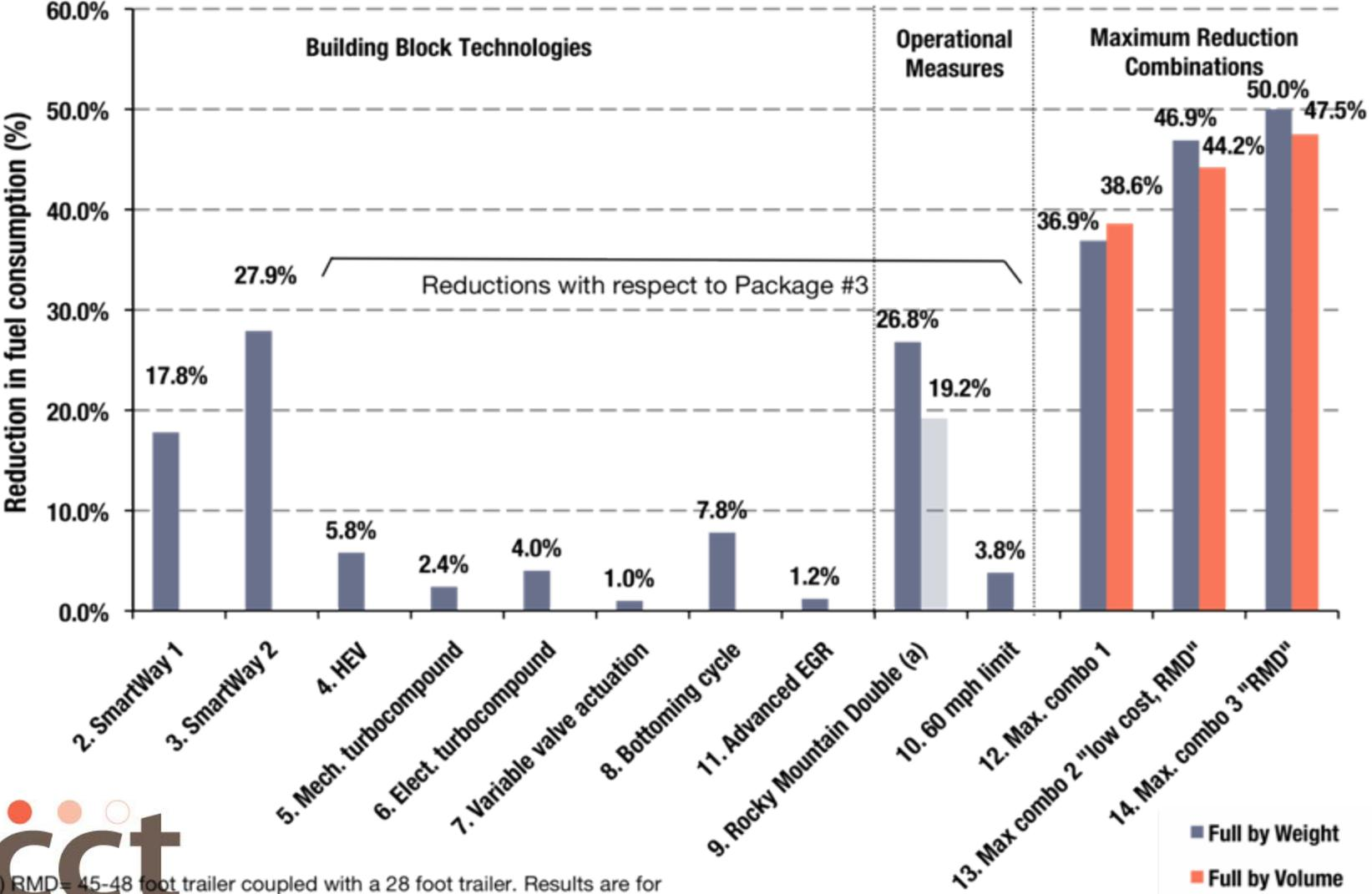
(a) RMD= 45-48 foot trailer coupled with a 28 foot trailer. Results are for freight density above 13,3 lbs.ft<sup>3</sup> and under 11.9 lbs/ft<sup>3</sup> respectively
