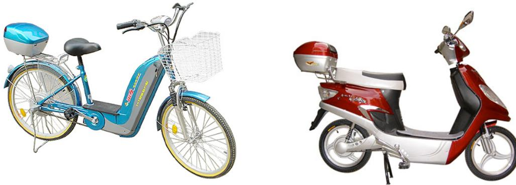
Figure 1: Bicycle Style and Scooter Style Electric Bikes
