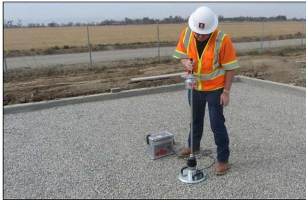
**Figure 3.2: Light weight deflectometer.**
