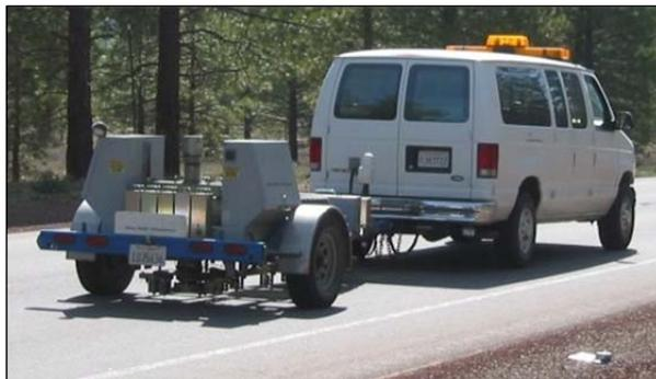
**Figure 3.1: Falling weight deflectometer.**
