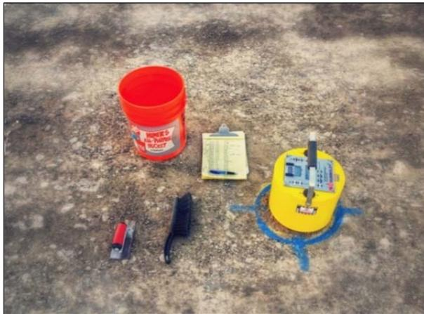
**Figure 3.3: Soil stiffness gauge.**
