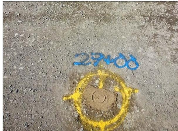
**Figure 3.4: SSG footprint in sand patch.**
